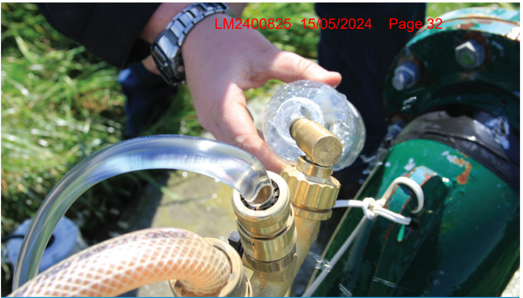
Taking a water sample at a wellhead
