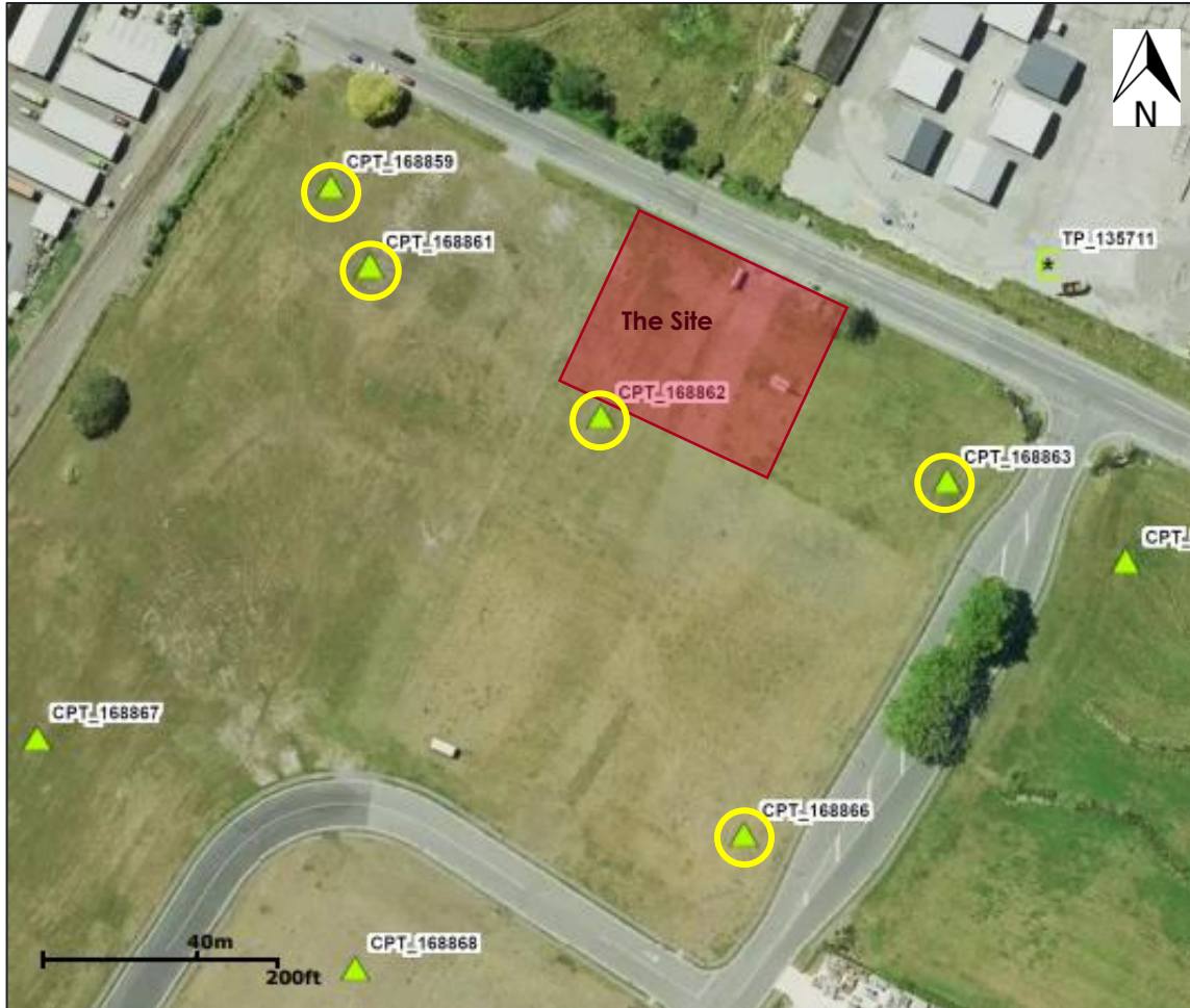
Figure 5. CPT locations from the NZGD whose data was used to analyse the liquefaction potential
