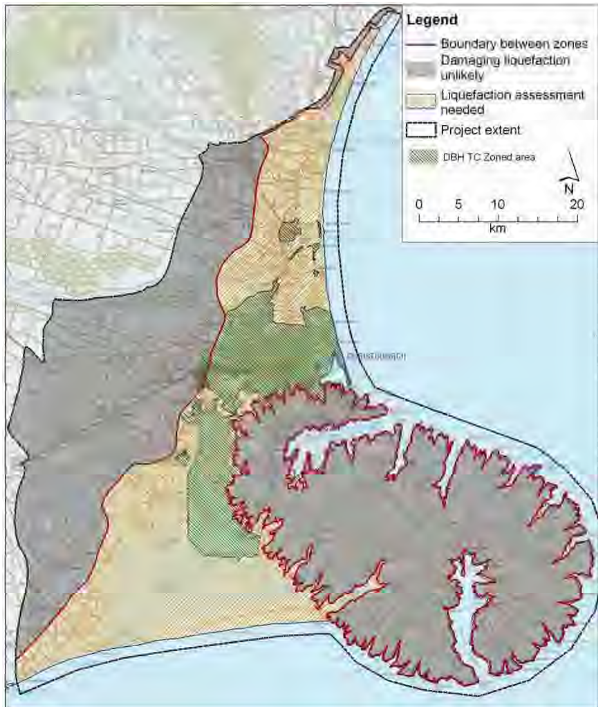
Figure 2.1 Liquefaction assessment area map for the eastern Canterbury project area. Liquefaction susceptibility is categorised in two areas, “damaging liquefaction unlikely” and “liquefaction assessment needed”. The area covered by DBH Technical Categories at the time of this report is excluded.
