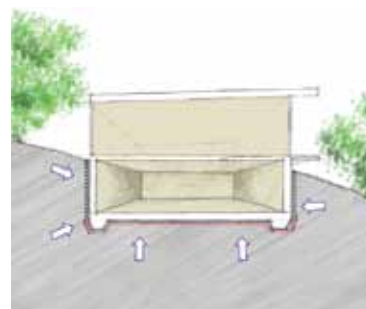
Cross-section of a fully encapsulated basement
