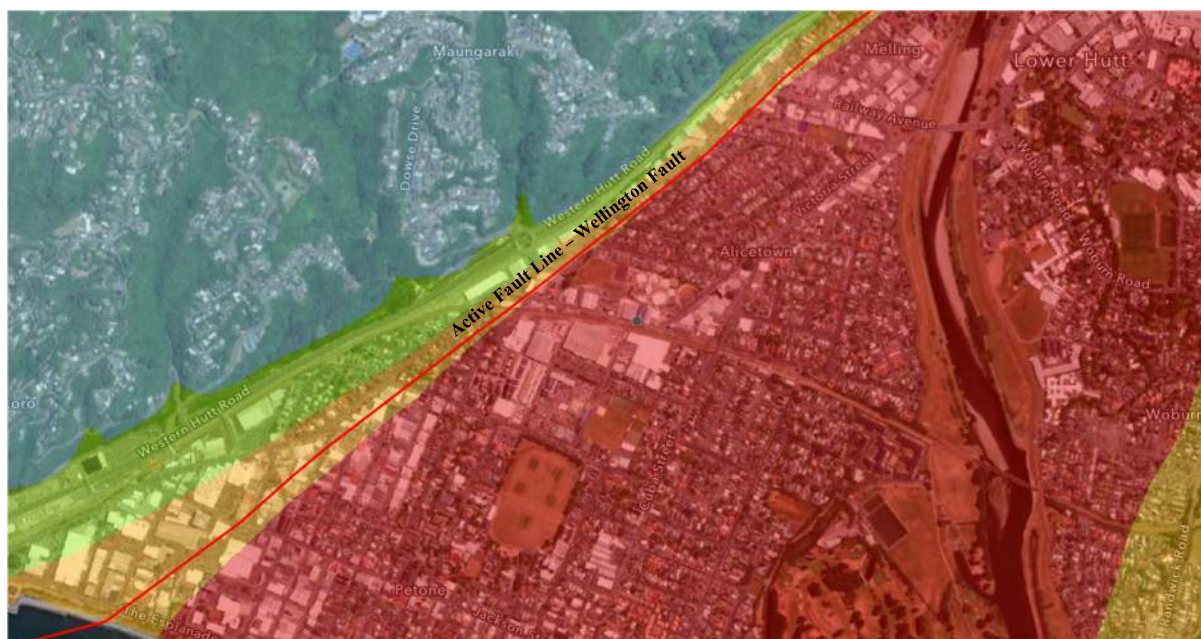
Figure 3. Ground shaking risk –High (GWRC webmap) and location of active fault (240m)
