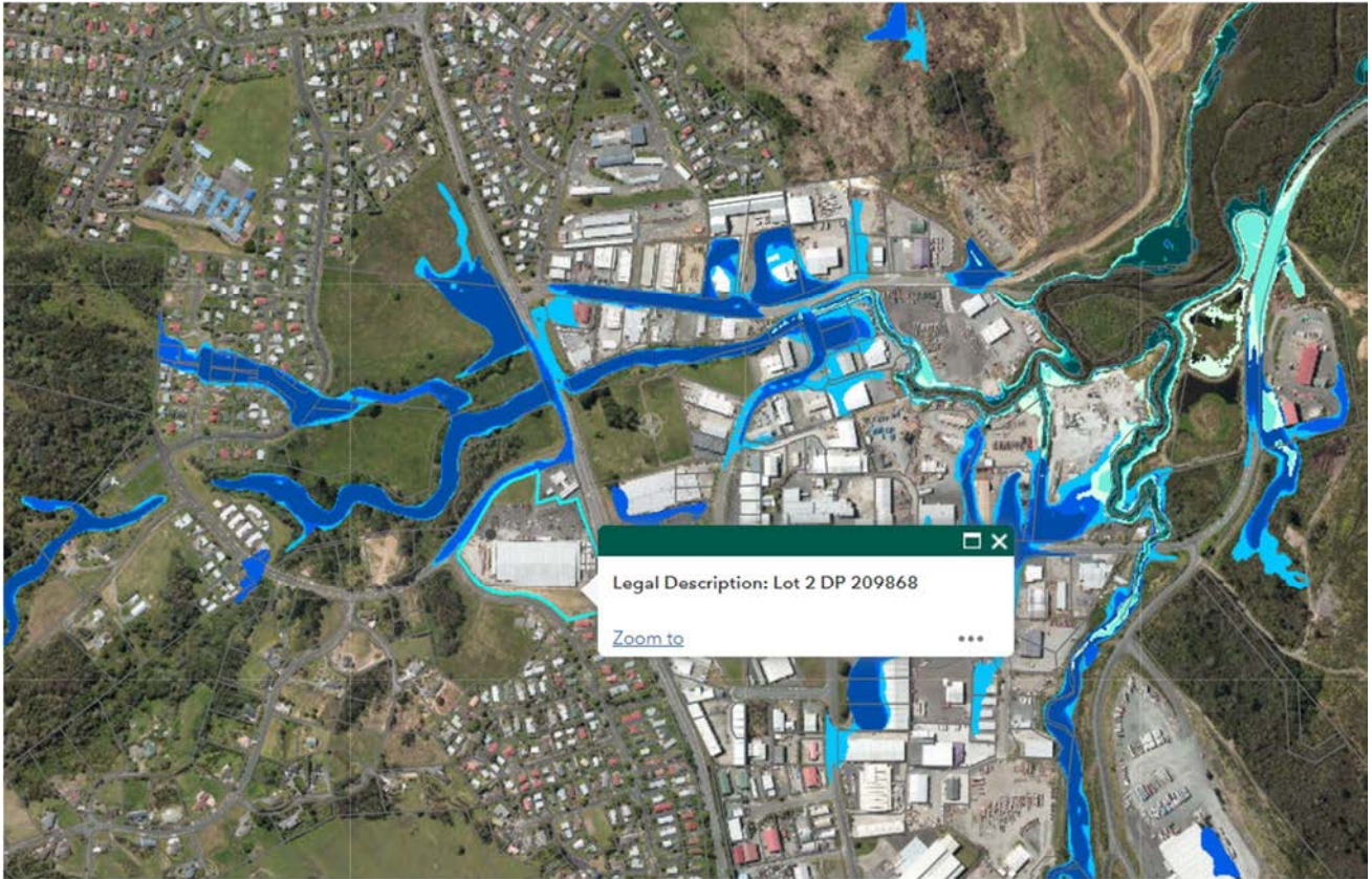
Figure 4 – Extents of the flood hazard areas downstream of the site. (NRC Hazard map)
