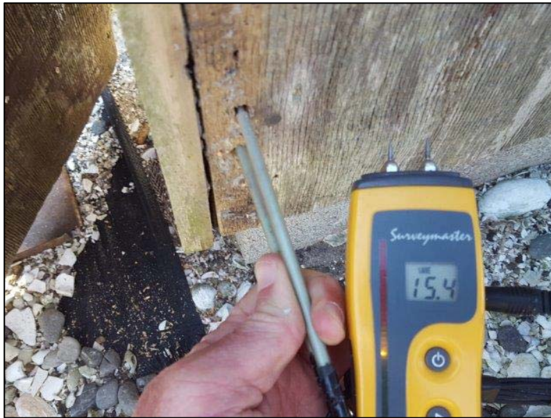
Photo 22: MC 15% normal moisture reading taken at workshop south corner. Ground clearance is approximately 200mm from floor slab to unfinished ground level (225mm required to meet Acceptable Solution). Refer Dodd drawings (Minor Alterations 2)
