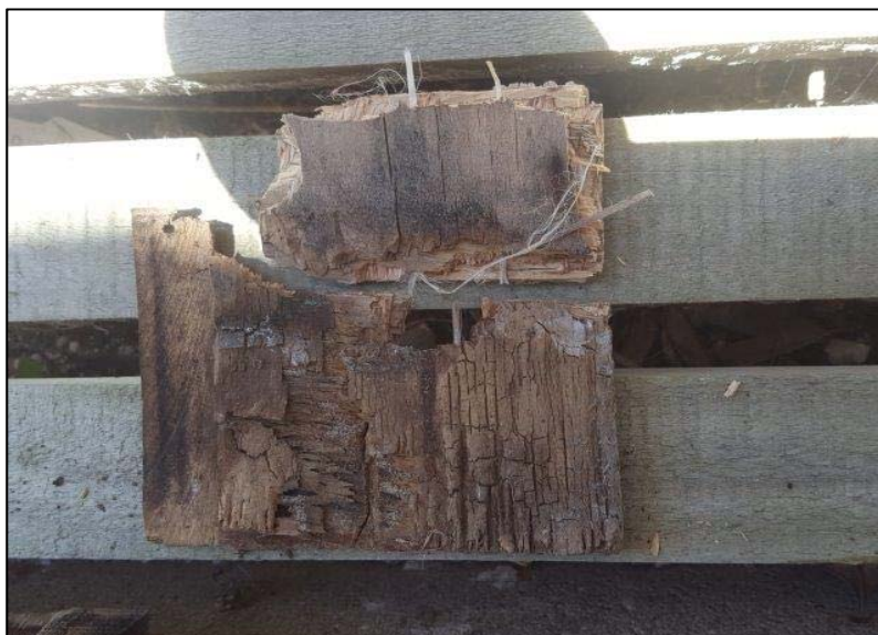
Photo 33: Visibly decayed cladding (rear face) from cutout. The Ecoply technical manual in 1999 stated that H3 treated plywood is not ground contact treated and must be kept at least 150mm away from ground contact
