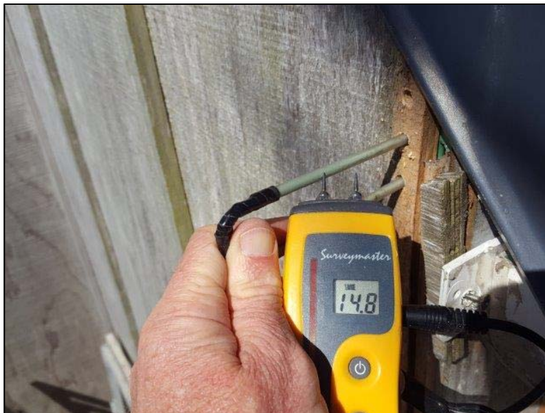
Photo 17: MC 14% normal moisture reading taken in framing at workshop external corner. Refer next photo
