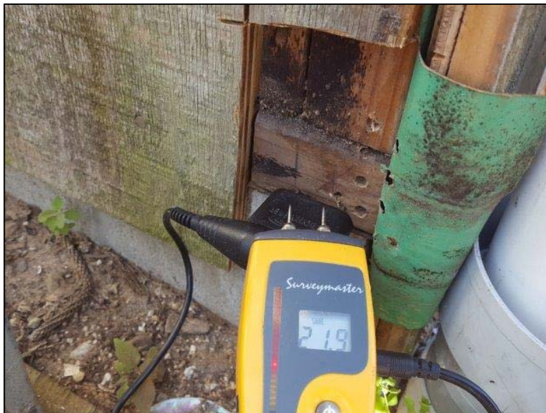
Photo 20: MC 21% elevated moisture reading at workshop external corner. Bottom plate is dark. No galvanised steel flashing was installed. Ground clearance is approximately 130mm from floor slab to unfinished ground level (225mm required to meet Acceptable Solution). Refer Dodd drawings (Minor Alterations 2)
