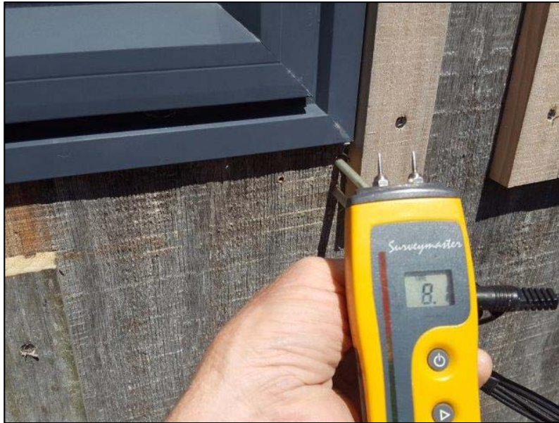
Photo 76: MC 8% normal moisture reading below sill flange
