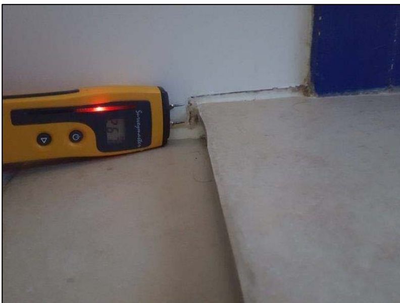
Photo 102: Moisture meter indicates elevated moisture levels on rear face of wall linings. It is assumed that undertile waterproofing will have been carried 150mm up behind the wall linings. There was no indication of any failure of the wall linings such as delamination. Refer following photos of flooring in adjacent space
