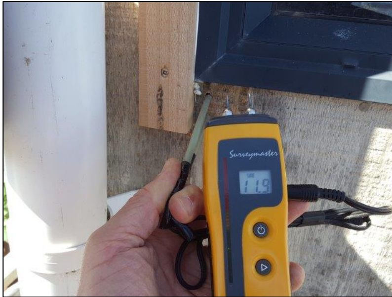
Photo 79: MC 11% normal moisture reading below sill flange. Drill shavings looked in good condition. MC 12% normal moisture reading was taken below sill flange at other end of window. Drill shavings also looked in good condition
