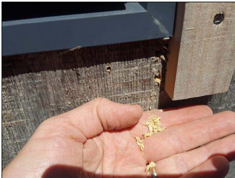
Photo 77: Drill shavings looked in good condition
