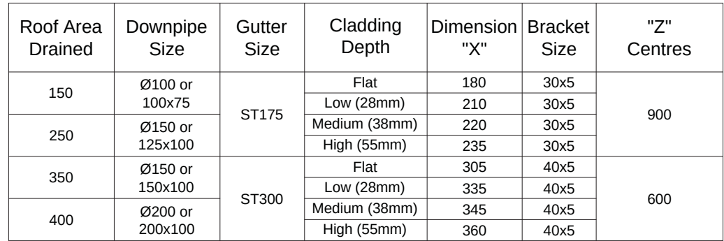
D. 01 TYPICAL GUTTER
