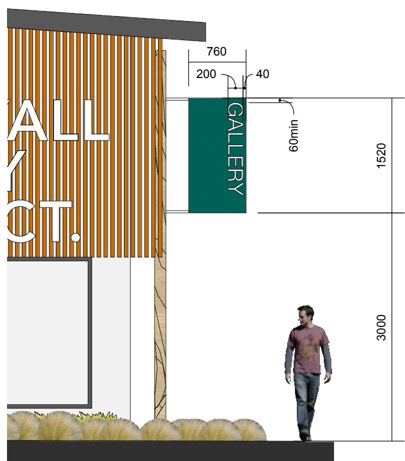
Banner flags mounted to timber pole
