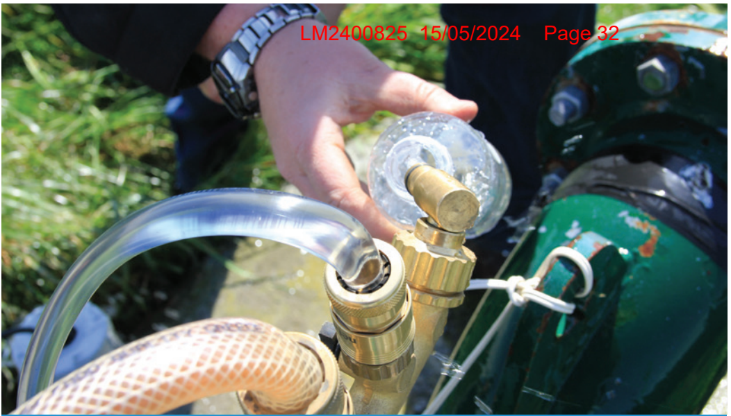
Taking a water sample at a wellhead
