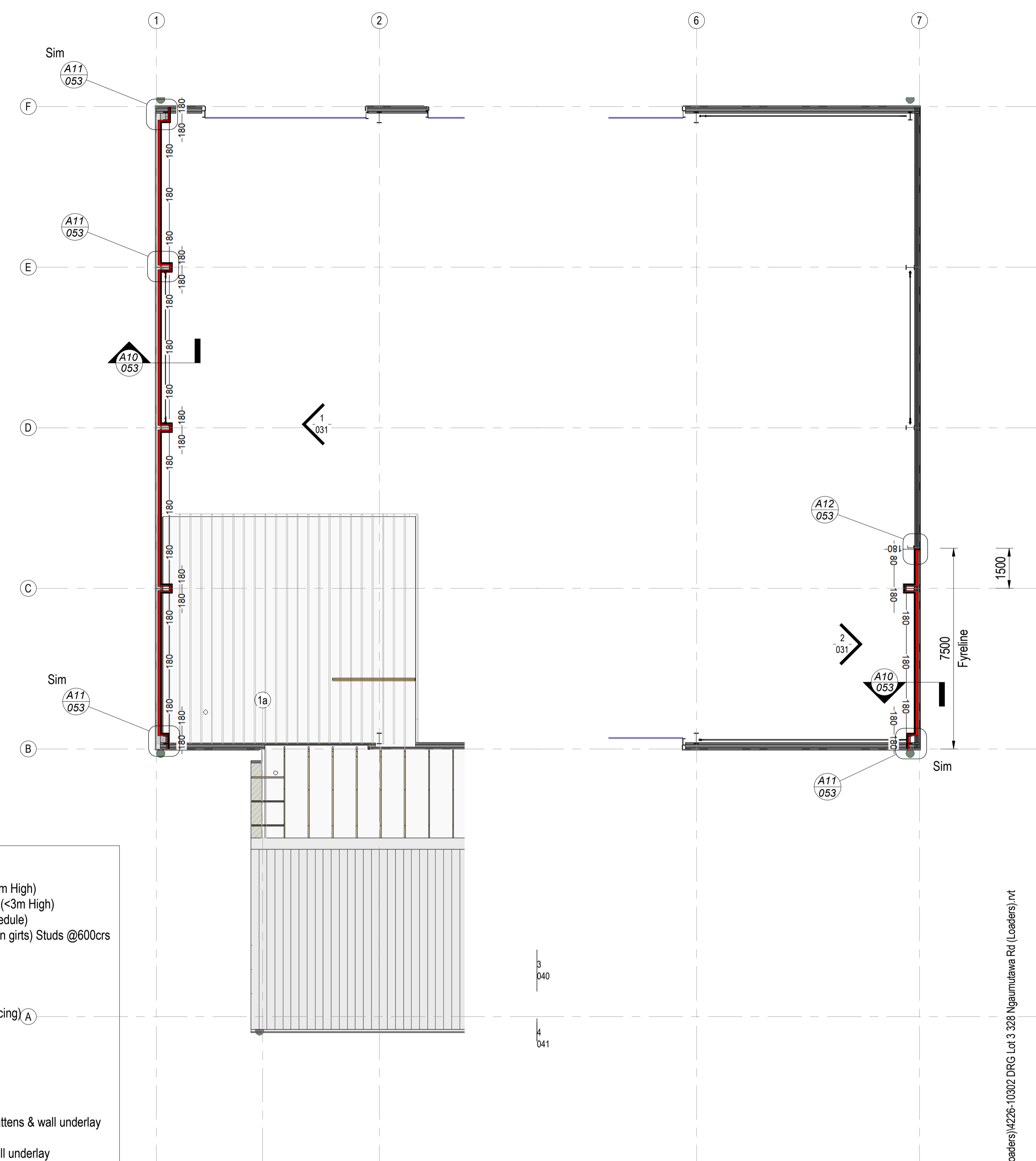
Wall Plan (Fire Walls @ RL +2400) 1:100 @ A1
