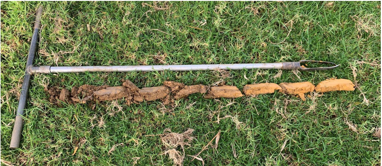
Photograph 2: Borehole showing 100mm of category 5, slightly moist, brown, clayey topsoil followed by category 6, slightly moist, brownish orange friable clay to a depth of 600mm. From 600-1200mm soils were orange clay.
